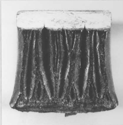
Figure 1.4: Parallel splits on the fracture surface of a transverse 3CR12 Charpy V-notch impact specimen. These splits developed in the rolling plane during impact testing.
