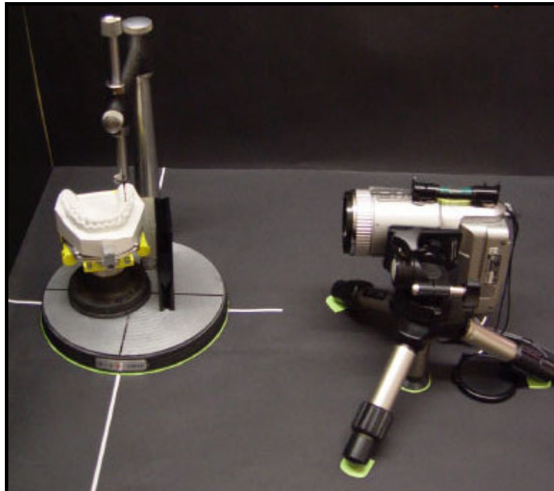
Figure 19: Complete photographic setup (side view)
