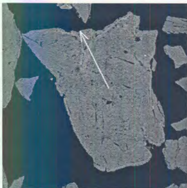
Figure 76. WDS Line chemical analysis through a particle of standard titania slag that was oxidised at 1050 °C for 60 min in 10 % O 2 .
