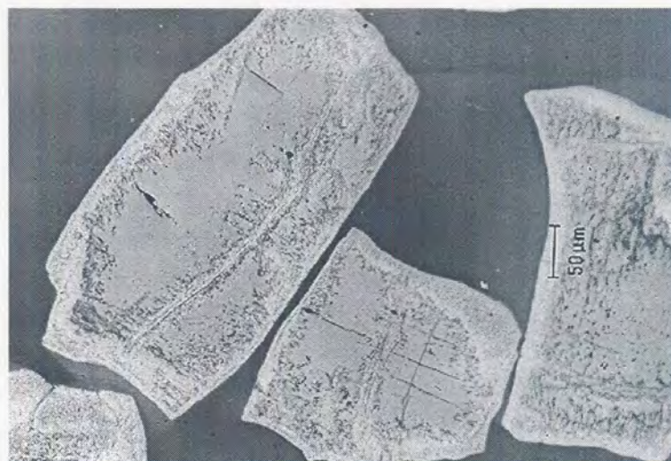
Figure 22. Optical micrograph of the high iron slag which was oxidised for 2 h at 850 °C, reduced for 30 min. at 800 °C, leached for 12 h and calcined. The exterior of the particles consisted predominantly of rutile and the interior predominantly of anatase.
