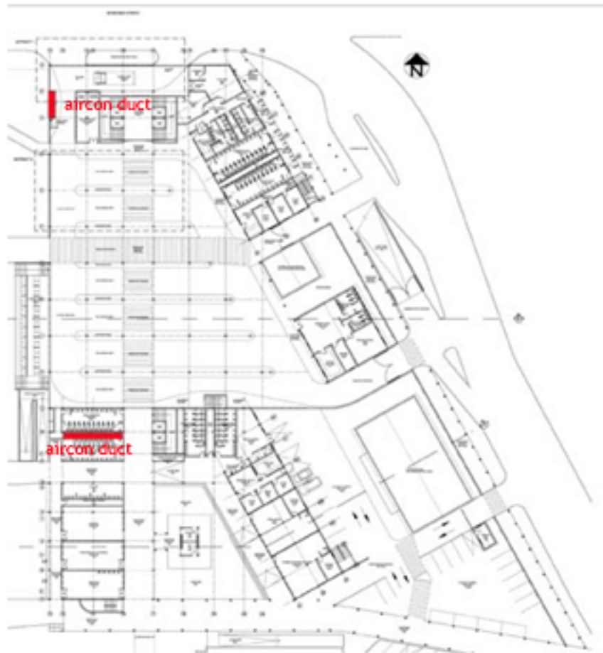
Positioning of Aircon ducts in subsequent floor levels
