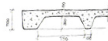
Typical coffered slab profile
