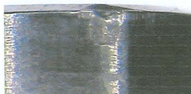
Figure 1.4: Worn turning tool insert
