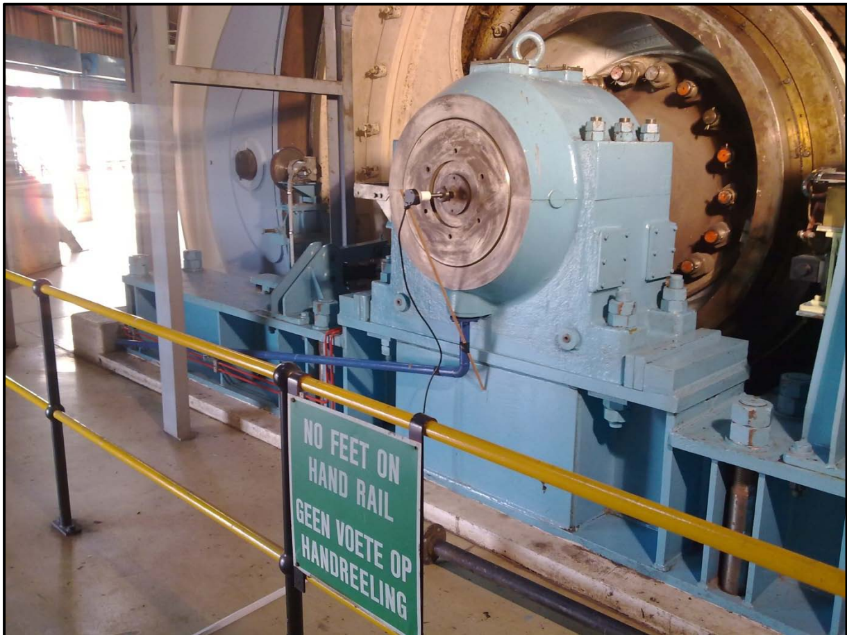
Figure 3-8: Rotary encoder connection on winder side shaft
