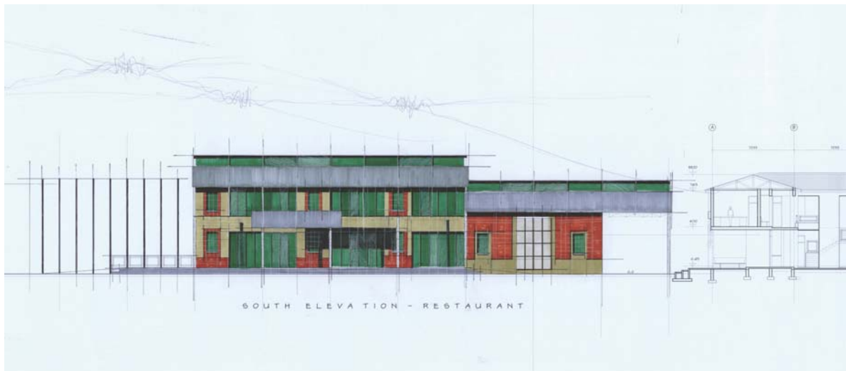
fig. [37] PROPOSED NEW RESTAURANT; SOUTH ELEVATION EXTERNAL FINISHES TO MATCH EXISTING AND PROPOSED ALTERATIONS TO THE NEW THEATRE
