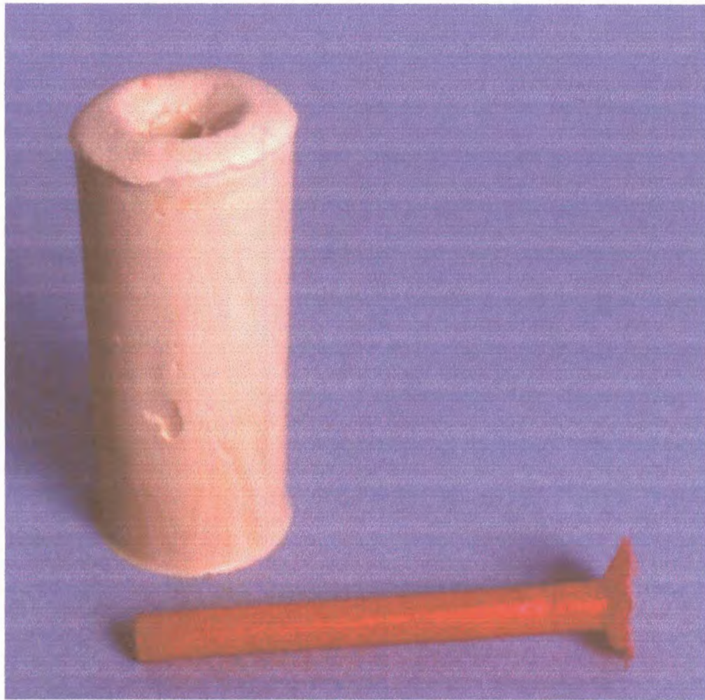
Fig 4-2: DuraLay resin rods as fabricated from the duplicating mould
