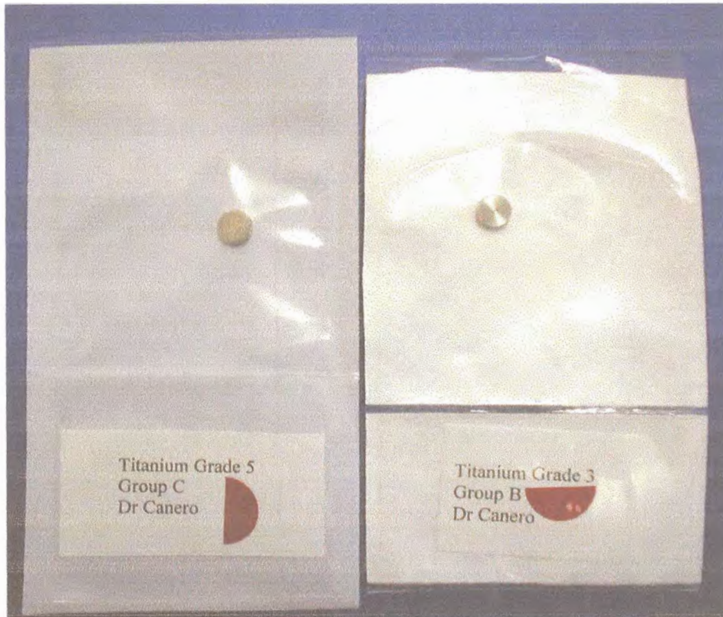
Fig 4-1: Sample discs of cpTi (Grade 3) and Ti6Al4V (Grade 5) as received from Southern Implants
