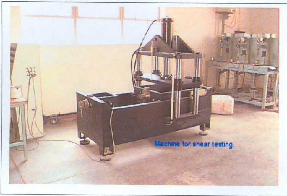
Figure 3.3 The large shear testing machine
