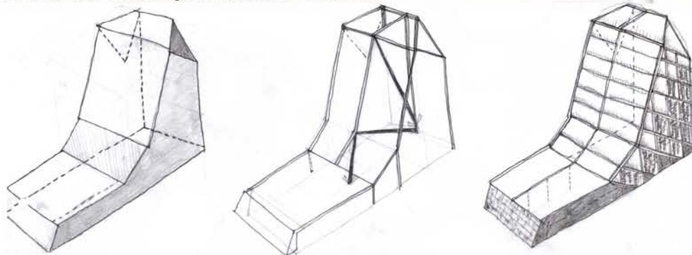
FIG 6.19 Spaceframe structure of stacked greenhouse idea - June 2008
