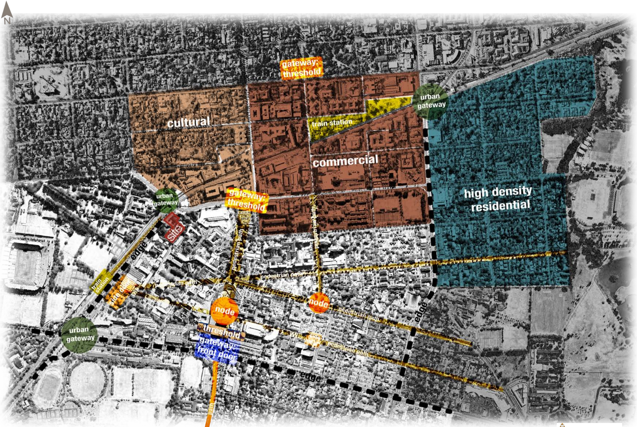
FIG 3.5 Alteration of the TOD proposal to allow for the university campus to integrate with the precinct over time
