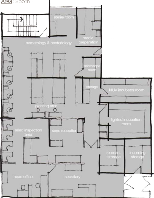
FIG 5.14 Layout plan of the main facility at Rajendranagar (Kahn 1999:39)
