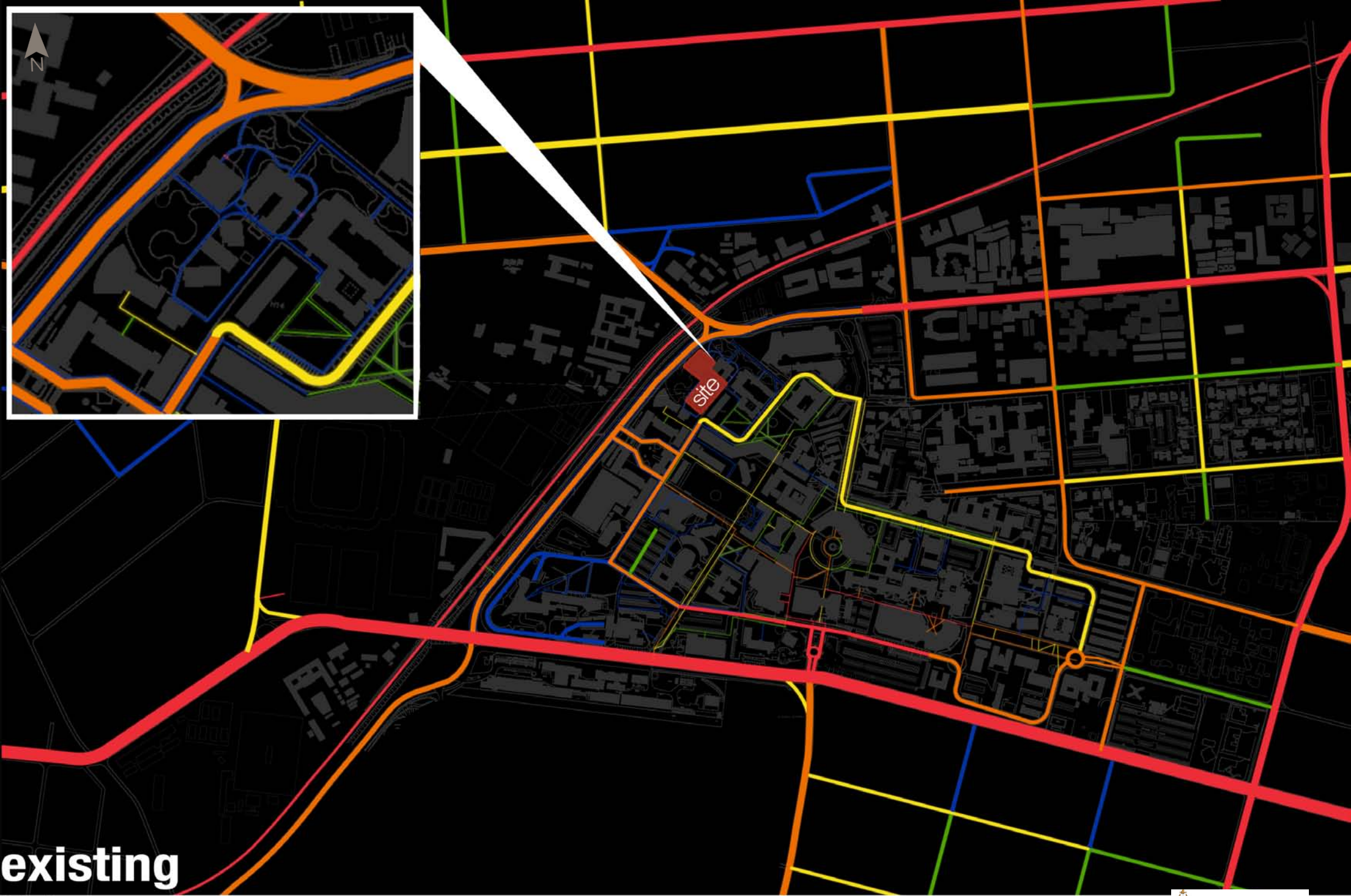
FIG 3.10 Space syntax diagram showing energy flows of cars and pedestrians on exiting campus and surroundings
