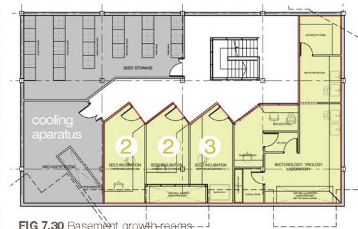
FIG 7.30 Basement growth rooms
