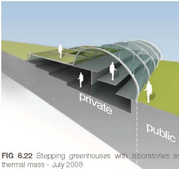
FIG 6.21 Stepping greenhouses with laboratories as thermal mass - July 2008
