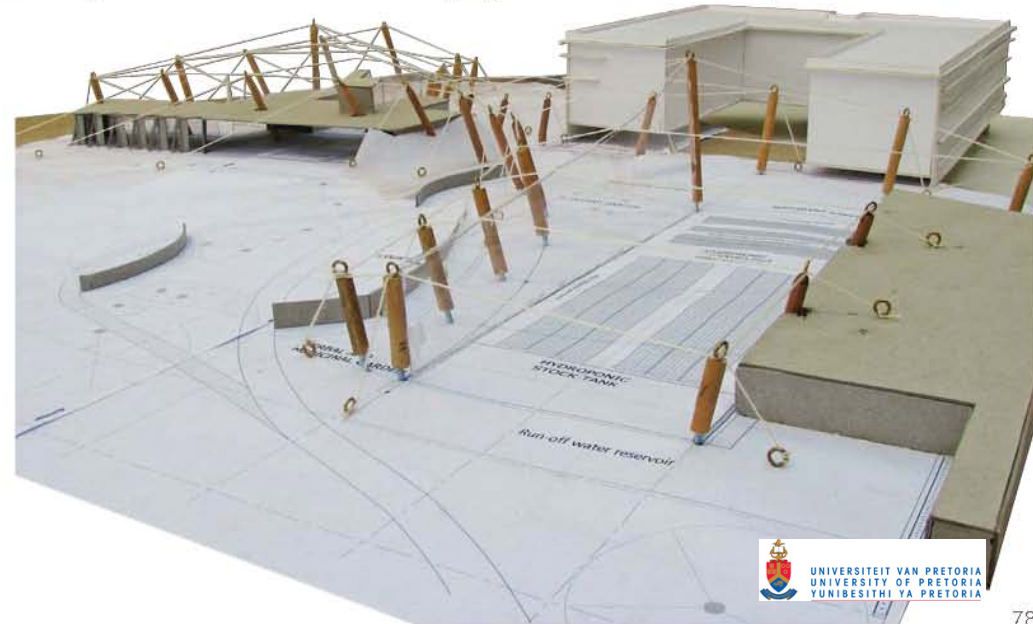
FIG 6.39-40 Final concept model using rope to imitate tensile members. This was used to determine the structural integrity of the assembly and the cohesion of the form language created with the site. September 2008
