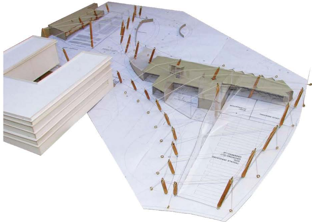
FIG 6.39-40 Final concept model using rope to imitate tensile members. This was used to determine the structural integrity of the assembly and the cohesion of the form language created with the site. September 2008
