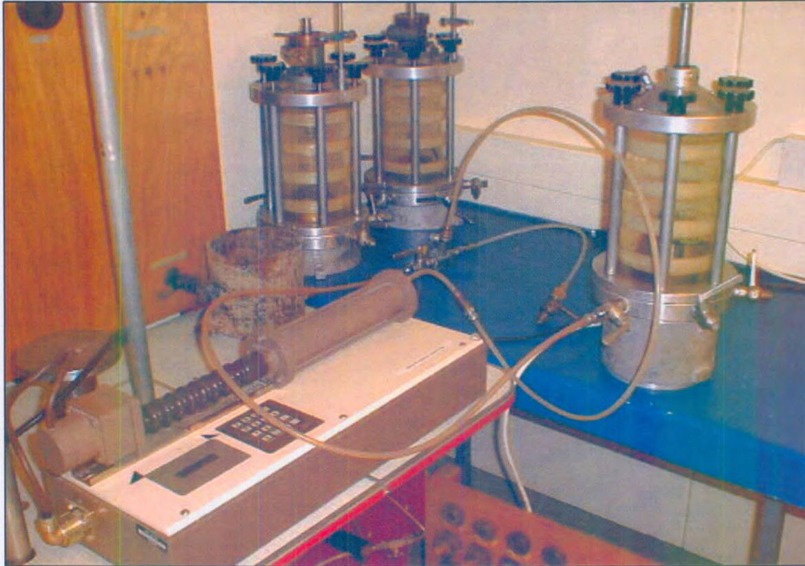
Figure 3.8: Saturation of the suction probe
