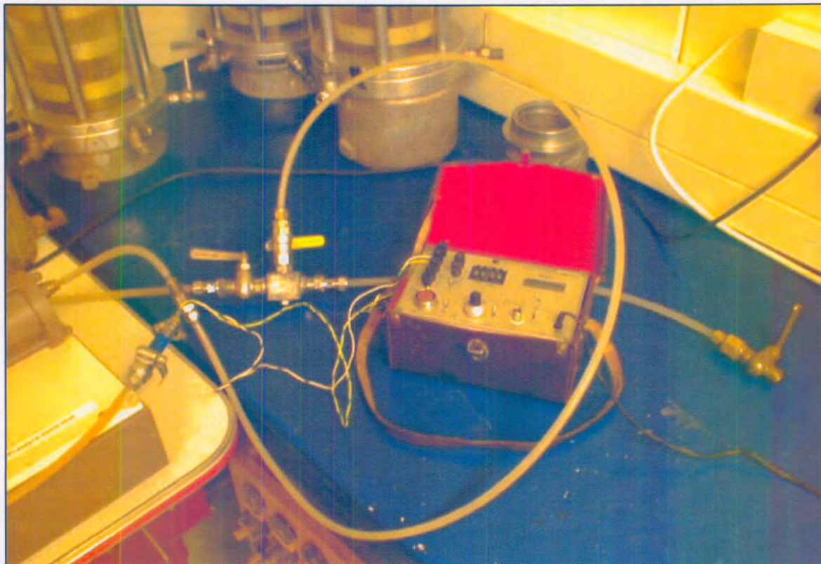
Figure 3.9: Calibration of the suction probe
