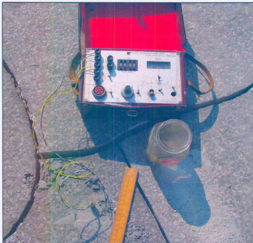
Figure 3.22: In-situ measurement of suction using the mid plane suction probe
