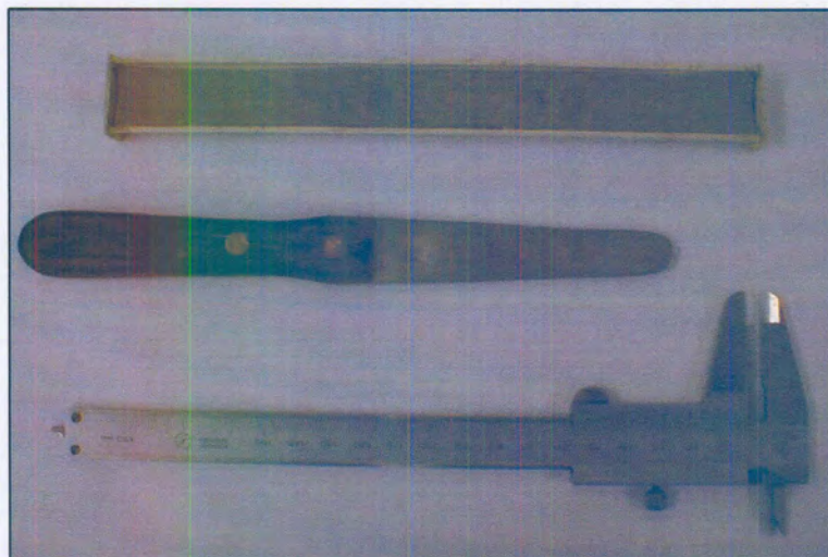
Figure 3.6: Tools used to measure volume change
