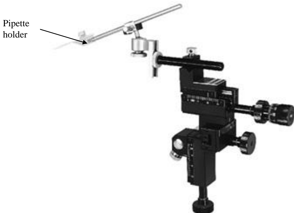
Figure 5.4: 152 Micromanipulator - a three dimensional coarse manual manipulator (The Narishe-Group).
