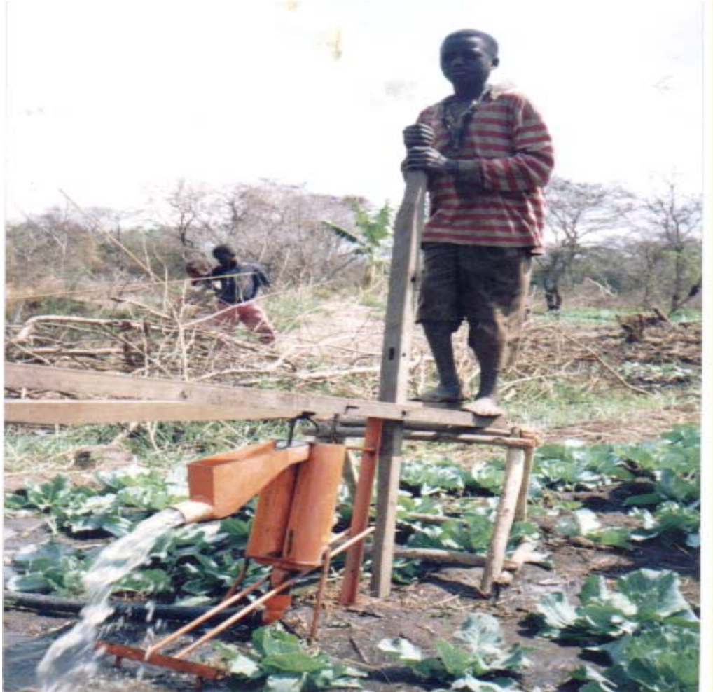
Figure 17: The modified well treadle pump superstructure.
