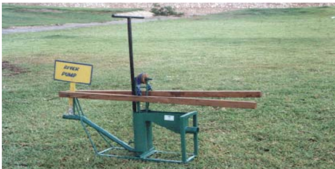
Figure 18: The river pump superstructure after installation.
