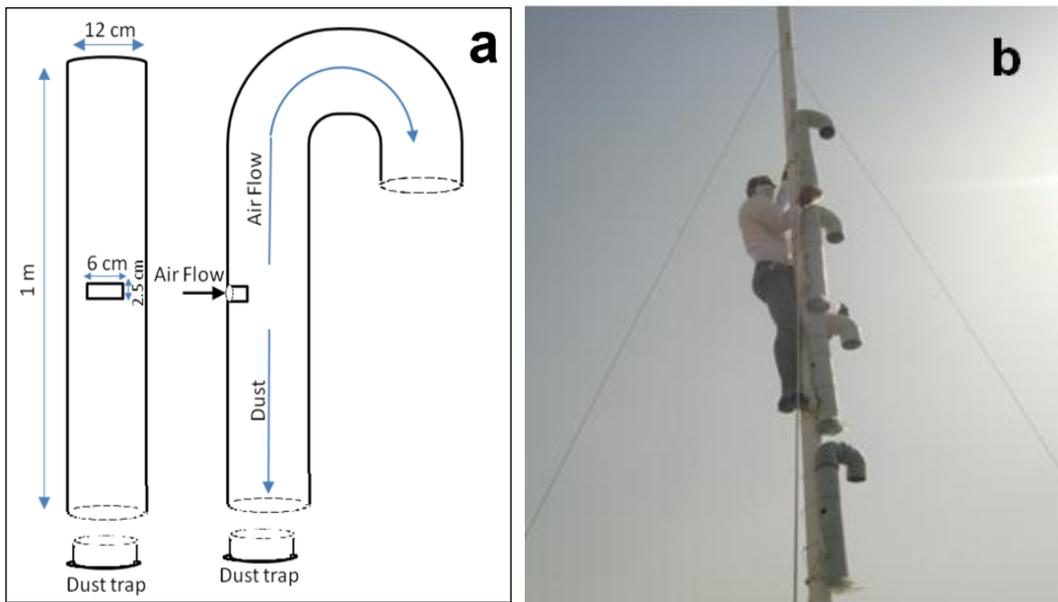
**Figure 3.9:** Schematic diagram of (a) the dust sampler system and (b) photo of the eight meters dust monitoring tower.
