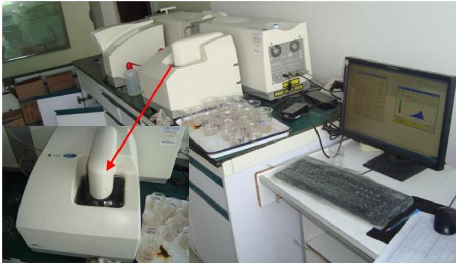
**Figure 3.10:** Measurement of dust particle-size using the Malvern Mastersizer 2000 analyzer (Lanzhou University, China).
