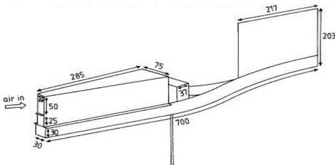
**Figure 3.1:** Construction of the Big Spring Number Eight (BSNE) sampler. Dimensions are in mm
