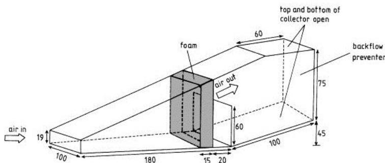
**Figure 3.4:** Sketch and construction scheme of the Wedge Dust Flux Gauge (WDFG) sampler. Dimensions is in mm
