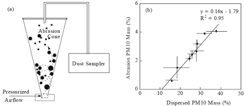
**Figure 3.7:** (a) A schematic illustration of an abrasion emitter; (b) Emission potential for PM10 for 8 soils plotted against the corresponding PM10 mass fractions determined using a dispersed analysis technique (Redrawn from Chandler *et al.*, 2002)
