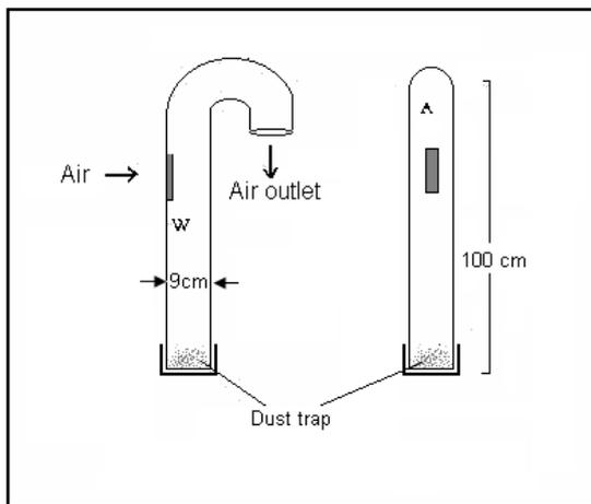
**Figure 3.5:** Construction of the Siphon Sand and Dust Sampler (SSDS) sampler
