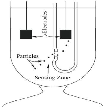
**Figure 3.6:** Illustration of the electrical sensing zone, showing an aperture tube immersed in an electrolyte with particles passing through the aperture (Redrawn from McTainsh *et al.*, 1997)
