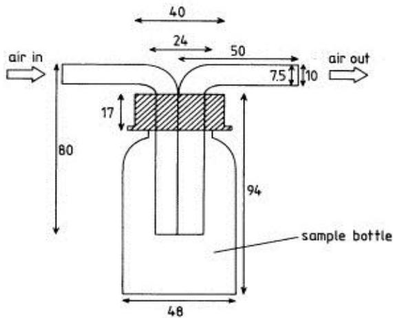
**Figure 3.3:** Sketch and construction of the Modified Wilson and Cooke (MWAC) sampler. Dimensions is in mm
