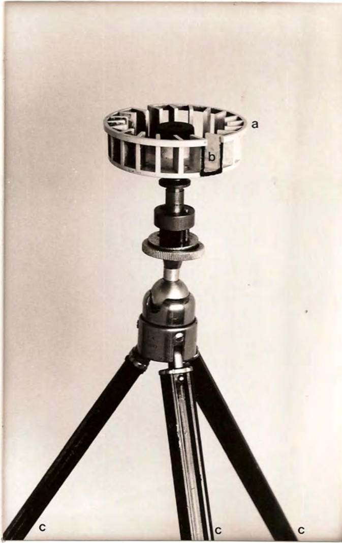
FIGURE 3.4. - A tripod-mounted, manual spinner for selecting consecutive plants in pairs, at random, in vegetation above the ground layer. a) spinner, b) sight, and c) telescopic tripod.
