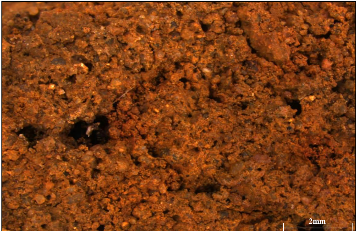
Figure 32: Optical microscope photograph - Unconsolidated Magaliesberg colluvium material (11.3x Magnification)
