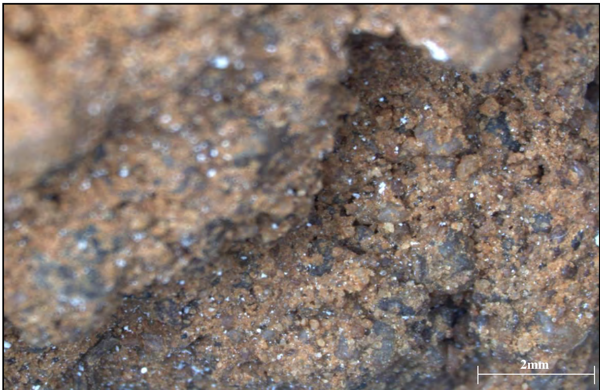
Figure 31: Optical microscope photograph - Consolidated Lephale aeolian sand (11.3x Magnification)
