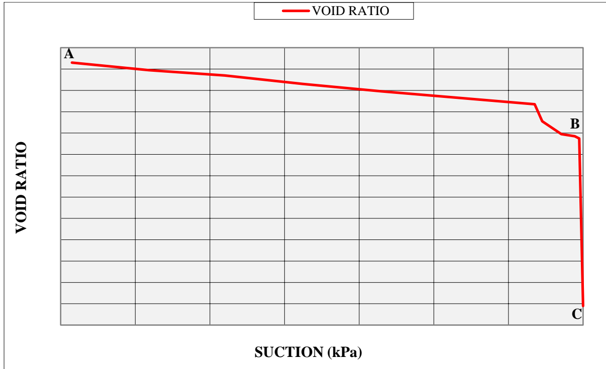
Figure 60: Two-phase behaviour between suction pressures and void ratio at a constant load of 200 kPa - Magaliesberg colluvium
