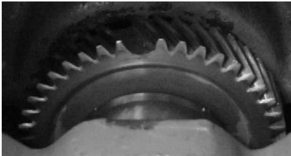
Figure 4.15: Damaged Drive Gear
