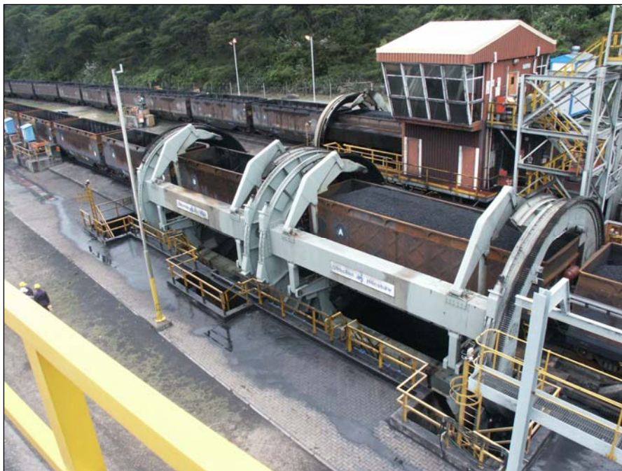
Figure 1.2: Tippler with wagons being pushed into position
