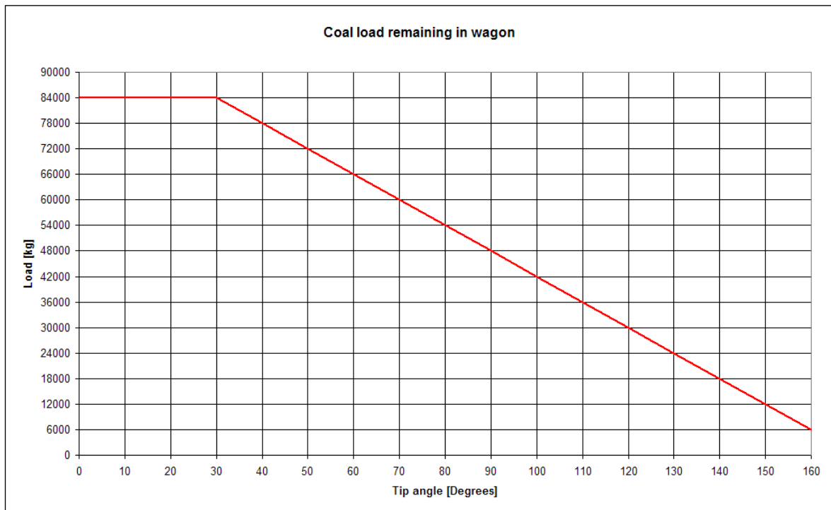
Figure 4.11: Coal weight in wagon for different tip angles
