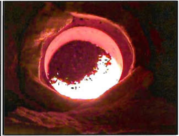
Figure 45: Establishing of a solids bed on top of the molten bath.
