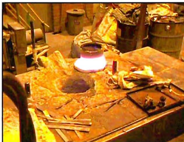
Figure 47: Crucible removed from the furnace for cooling.
