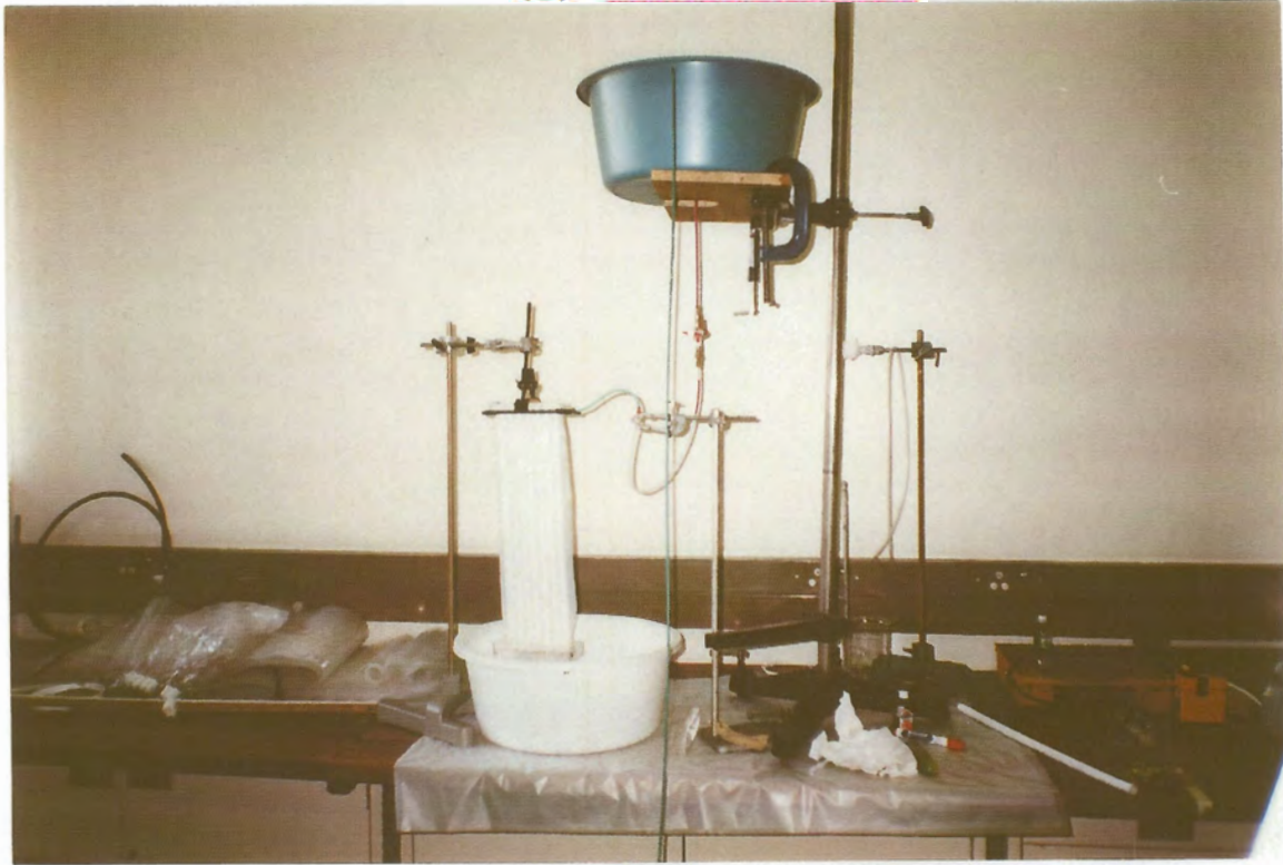
Fig.6.3 Experimental setup for wettability test.
