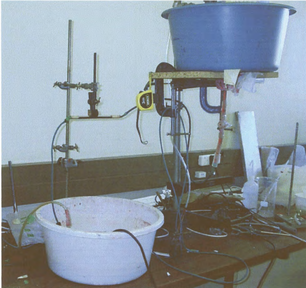
Fig. 6.17 Setup for liquid distributor testing.
