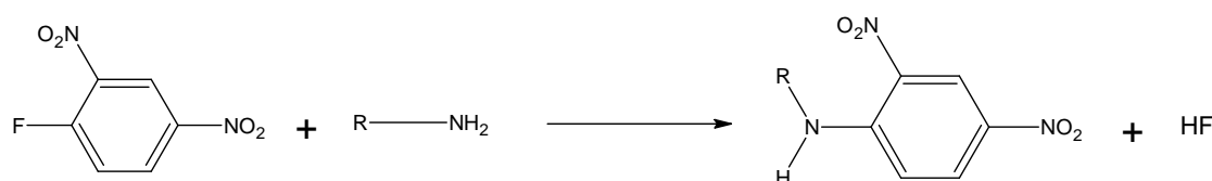
Figure 3.18 Reaction scheme for the reaction of 2, 4-dinitrofluorobenzene (DNFB) with a primary amine. R = alkyl or aryl substituent [121].
