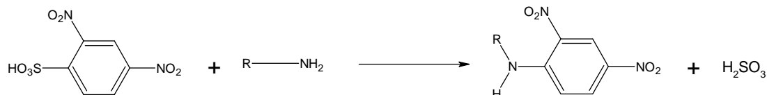
Figure 3.19 Reaction scheme for the reaction of 2, 4-dinitrobenzenesulphonic acid (DNBS) with a primary amine. R = alkyl or aryl substituent [121].
