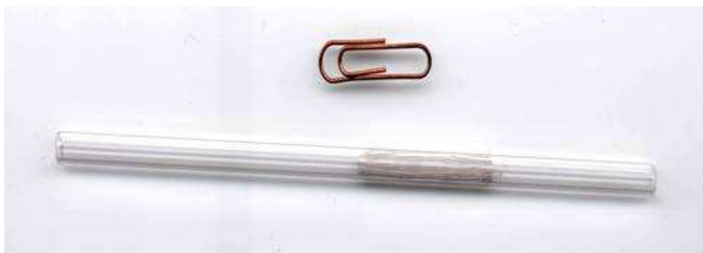
Figure 2.9 A polydimethylsiloxane multichannel trap (PDMS MCT). This trap has 32 x ~2 cm lengths of PDMS tubes arranged in parallel inside a glass tube. This shorter arrangement is suitable for trapping less volatile analytes which require longer desorption times.
