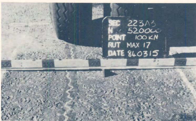
(c) Longitudinal crack on SECTION 1.
