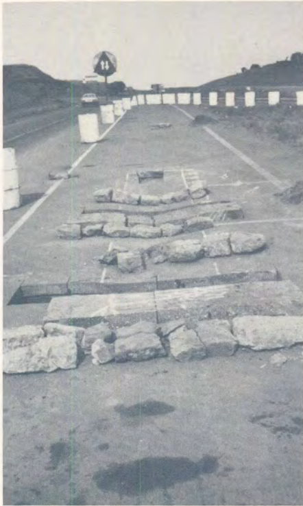
(a) Cross Profiles made across Section 1 after HVS trafficking. NOTE the deformation and recovered stabilized Berea Red subbase material (cracked).
