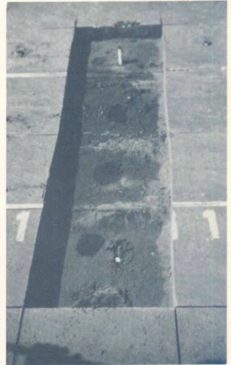
(d) Phenoltalien indication of relative high pH on the top of the upper subbase and the pumped layer.
