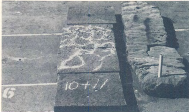
(a) Fatigue cracking at the bottom of the asphalt base layer after the EPWP state on Section 2.
