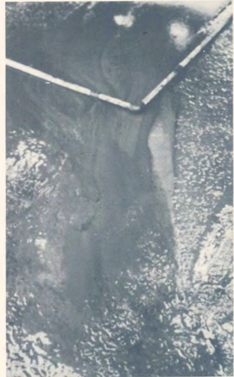
(b) Pumping from upper subbase during the wet test.
