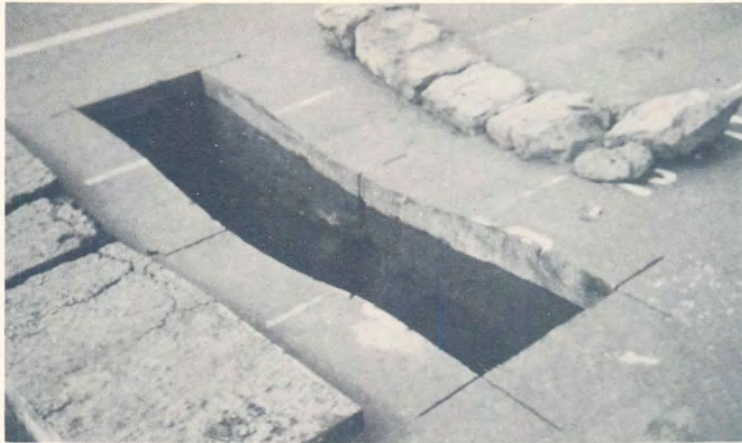
(a) Cross profile after EPWP on Section 2. Note the thinner subbase inside the trafficked area.
