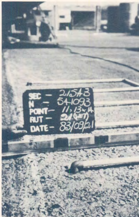
(c) 21 mm of permanent deformation (rut) on wet section. E80s on wet test section: 0,8 \times 10^6 .
