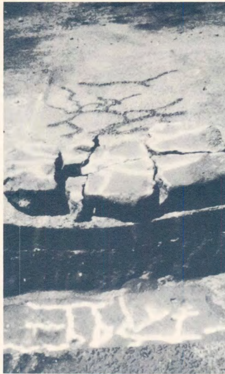
(a) Recovered cracked lower stabilized subbase layer within the trafficked area after the test. (Blocks on top of asphalt)
