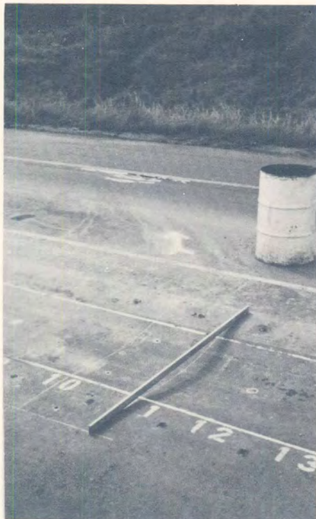
(b) Real road failure next to Section 2 in the normal trafficked lane during the time of HVS testing on Section 2.
