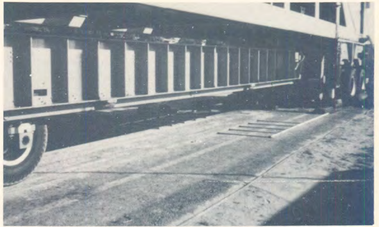
(b) General view of test on SECTION 1. Note the water inlet pipes on the side of the test section.
