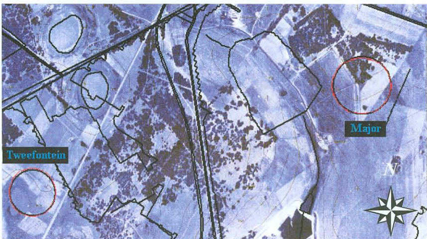
Fig. 5: Digital vector of the project pivots on Kleinkopjé Mine, overlaid to an aerial photograph (no scale available)
