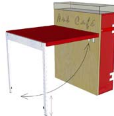
3 folding down table legs & adjusting leg height
