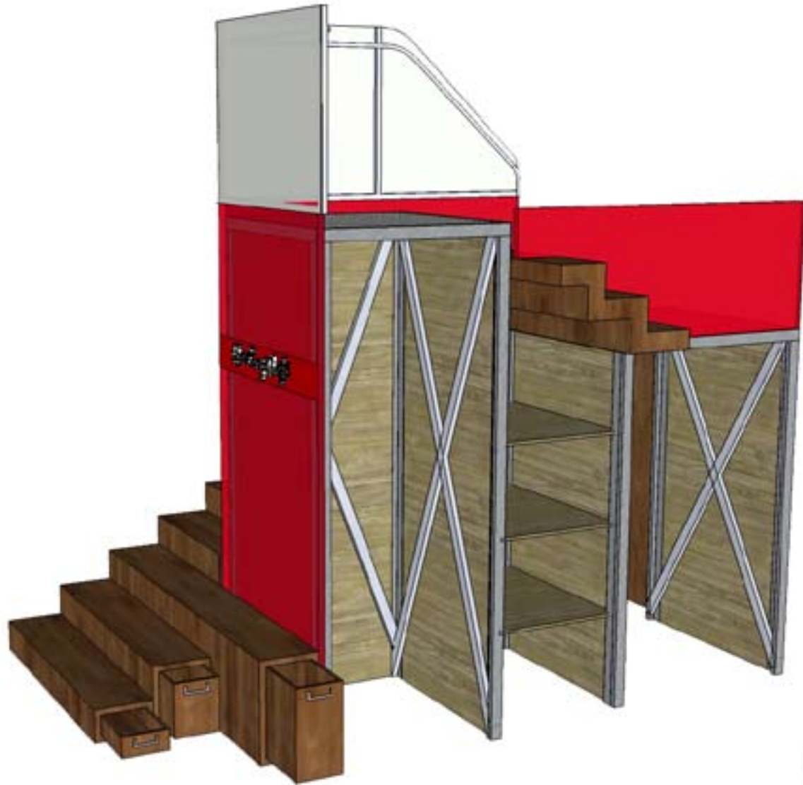
Figure 89(b): Back of staircase, showing storage facilities
