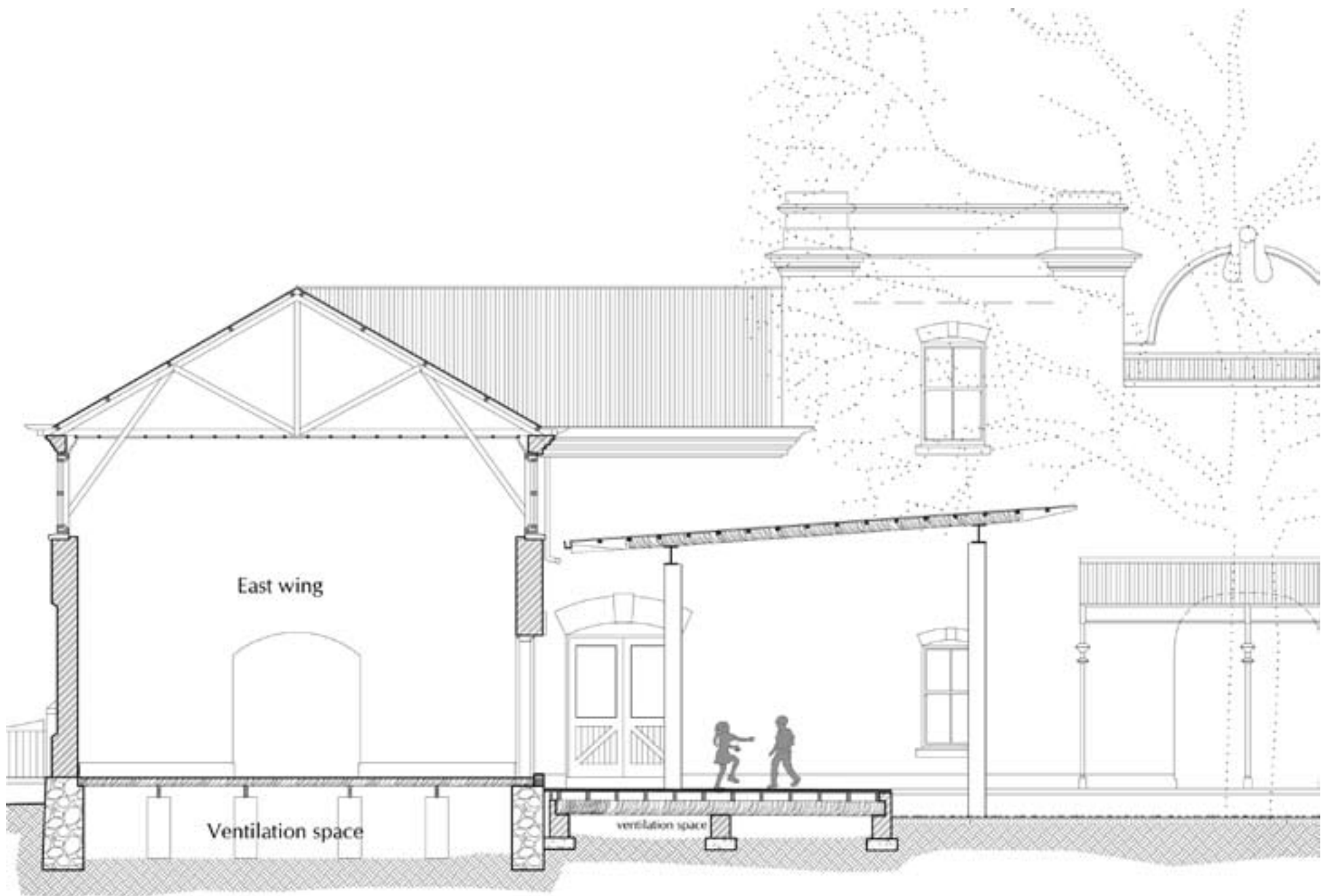
Figure 114: Detailed Section through the east wing and Pavilion Roof
