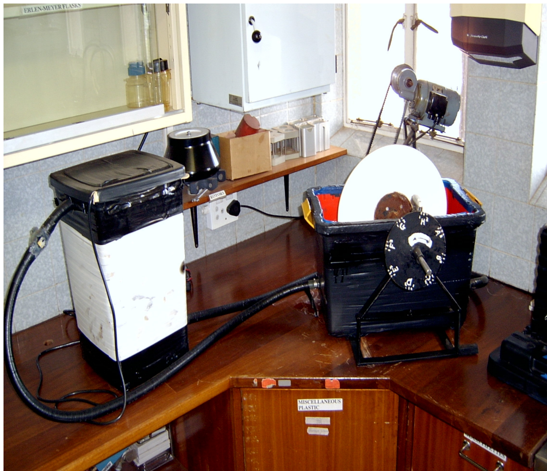
Figure 3.1 A biological rotating contactor used to monitor light reflectance
