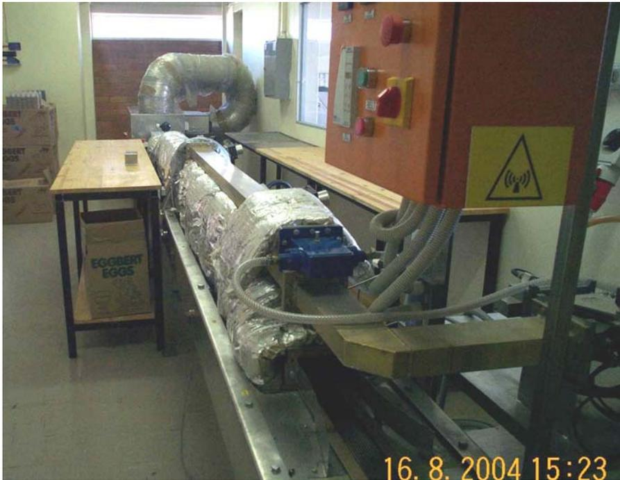
Figure 5. Prototype pilot-plant microwave oven unit. The conveyor belt is visible in the front, and two rows of eggs were packed in this continuous system.
