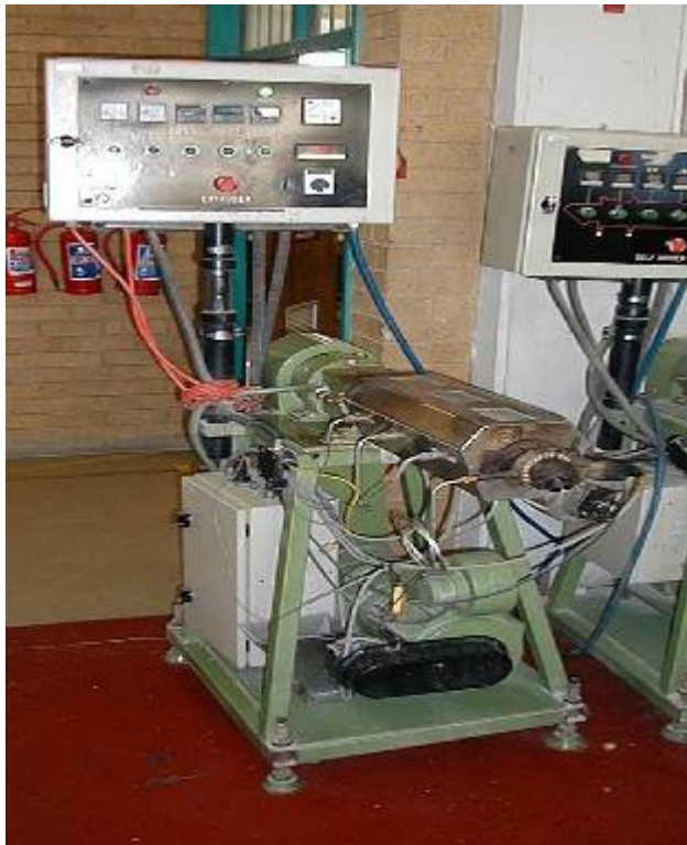
Figure 11: Rapra single-screw extruder
