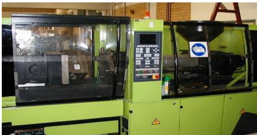
Figure 12: Engel 3040 screw-type injection moulder
