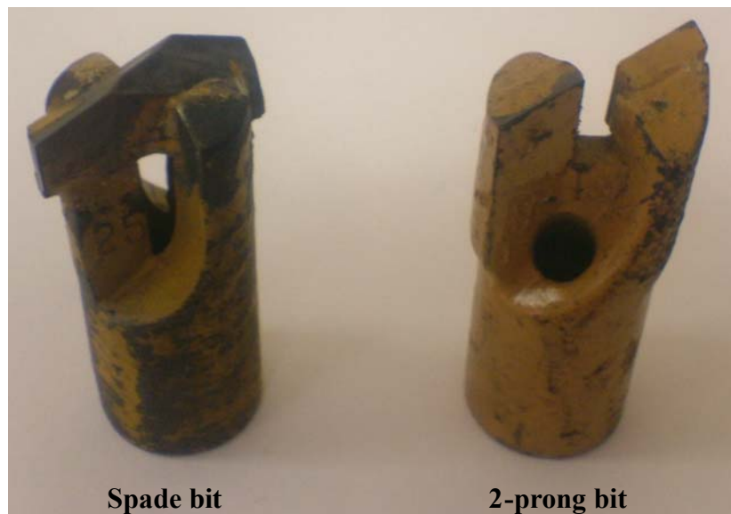
Figure 6-44 Spade and 2-prong bits (25 mm)
