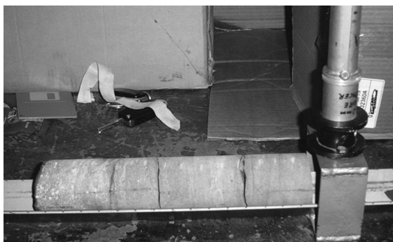
Figure 5-6 A fine to medium grained sandstone or “grit” unit after impact splitting, taken from borehole ARN 4968
