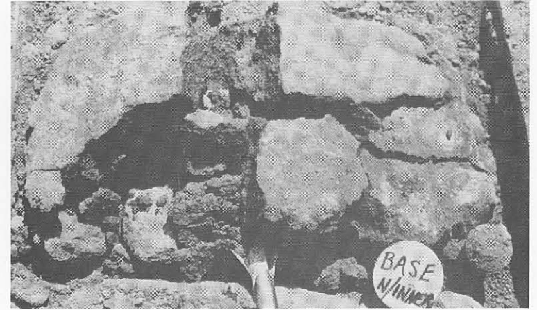
(a) Progress of both horizontal cracking and crushing of the top 50 mm to 75 mm of the cemented base after HVS testing.
