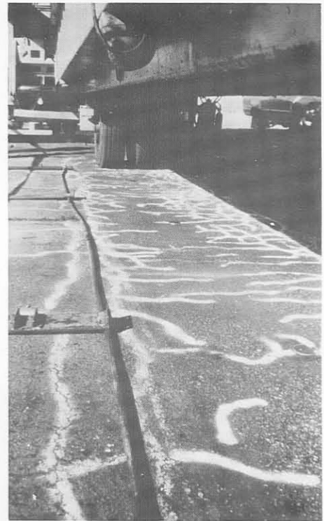
(a) Relatively fine cracking after 1,44 \times 10^6 100 kN repetitions.
