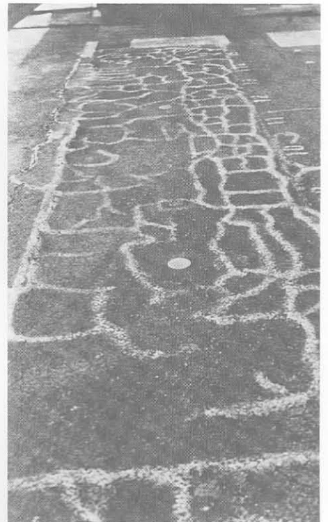
(b) Final fatigue cracking and crushing after approximately 2,64 \times 10^6 100 kN repetitions.
