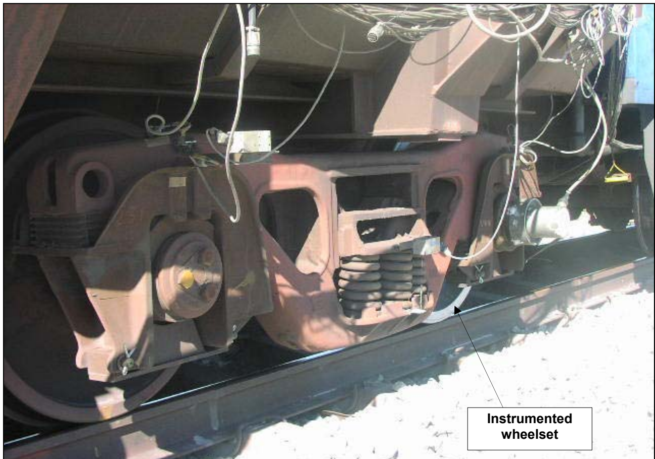
Figure 4-17: Instrumented wheelset installed in 30t per axle iron ore wagon
