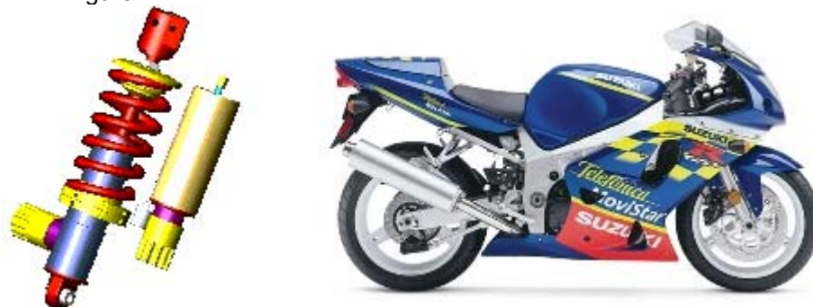
Figure 1-4: A CAD drawing of a racing motorcycle suspension unit developed for a Suzuki GSXR-600
