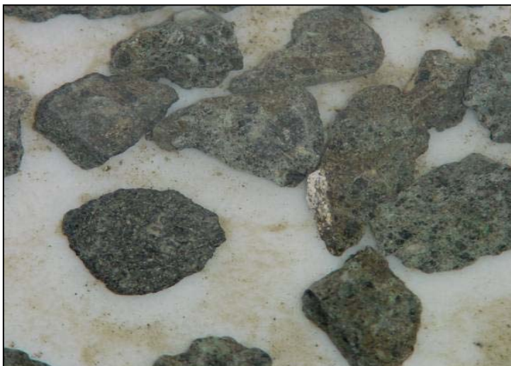
Figure 41. Visual appearance of Dutoitspan ore (initial size - 26.5 + 22.4 mm) weathered in ammonia chloride solution (0.4 M) for 6 days.
