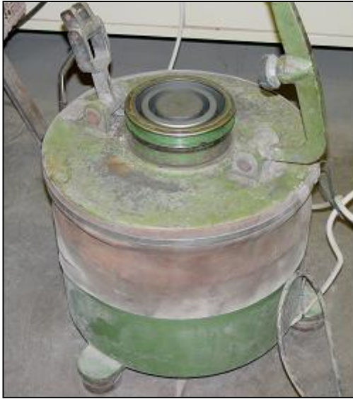
Figure 18. Swing mill used for agglomeration tests.
