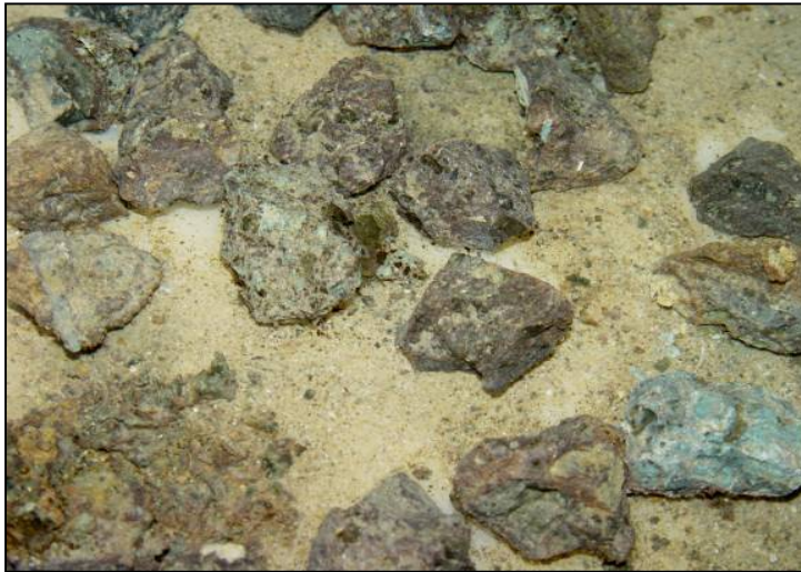
Figure 36. Visual appearance of Geluk Wes ore (initial size - 22.4 + 19 mm) weathered in aluminium chloride solution (0.2 M) for 6 days.
