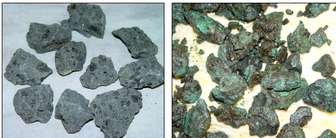
Figure 77. Venetia K2 South kimberlite unweathered (left) compared to the weathered product (right). Weathering was done in a 0.05 M cupric sulphate solution for 6 days.
