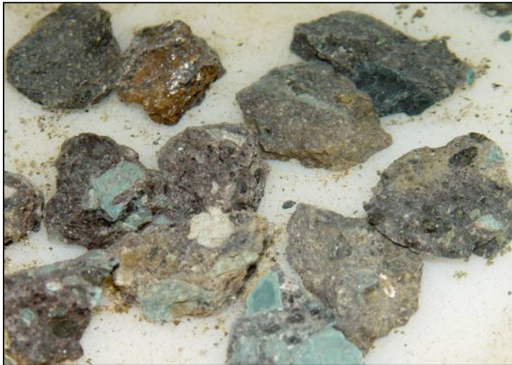
Figure 35. Visual appearance of Geluk Wes ore (initial size -22.4 + 19 mm) weathered in sodium chloride solution (0.2 M) for 6 days.
