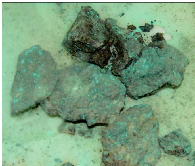
Figure 61. Visual appearance of Dutoitspan ore (initial size -26.5 + 22.4 mm) weathered in a 0.005 M cupric sulphate medium for 6 days.
