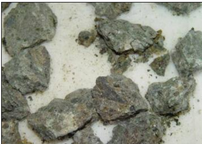
Figure 47. Visual appearance of Dutoitspan ore (initial size - 26.5 + 22.4 mm) weathered in magnesium chloride solution (0.4 M) for 6 days.
