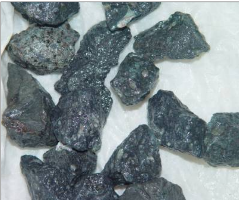
Figure 29. Visual appearance of Wesselton ore after the standard weathering test (- 19 + 16 mm).
