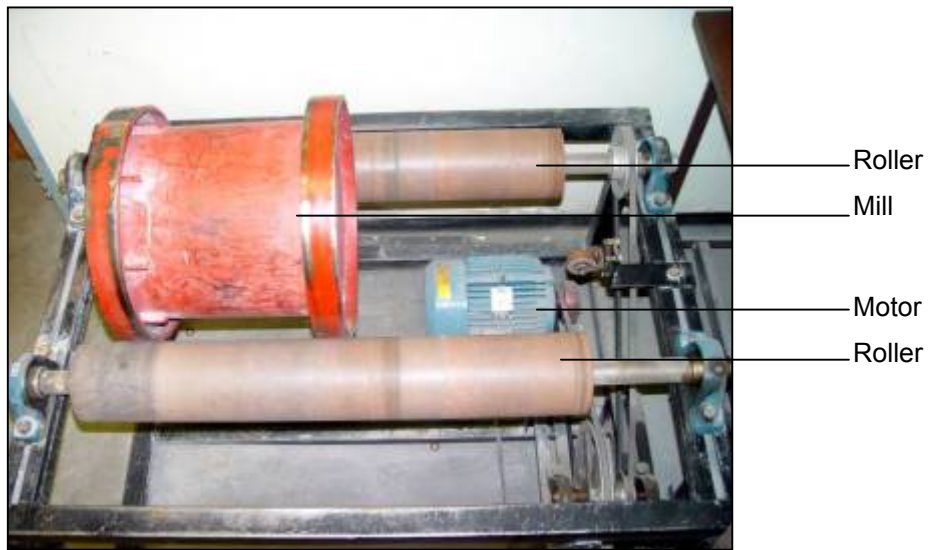
Figure 17. Autogeneous batch mill used.
