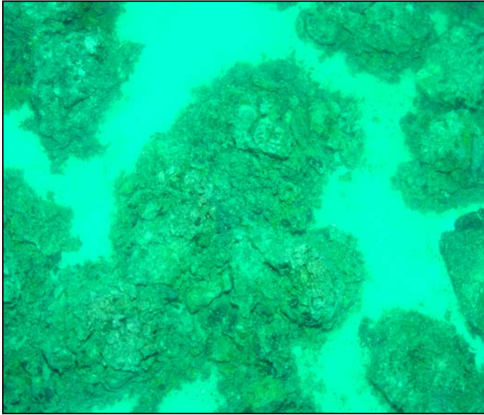
Figure 63. Visual appearance of Dutoitspan ore (initial size -26.5 + 22.4 mm) weathered in a 0.4 M cupric sulphate media for 6 days.
