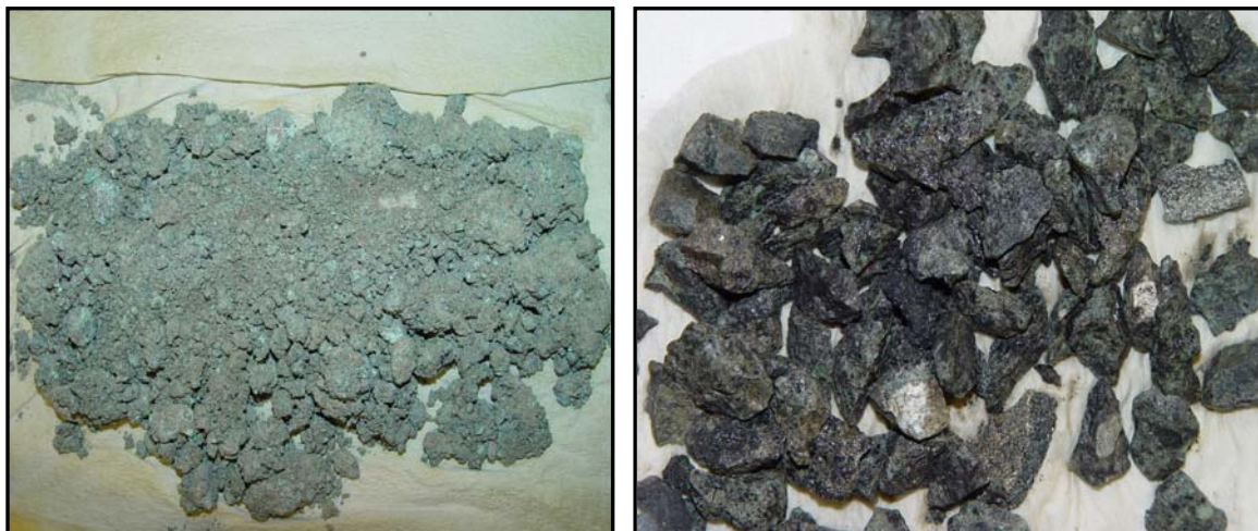
Figure 73. Comparison of the effect of copper (swelling cation) on the left and potassium (stabilising cation) on the right and their effect on the weathering of kimberlite (photos taken after 6 days for potassium and 15 days for copper medium).
