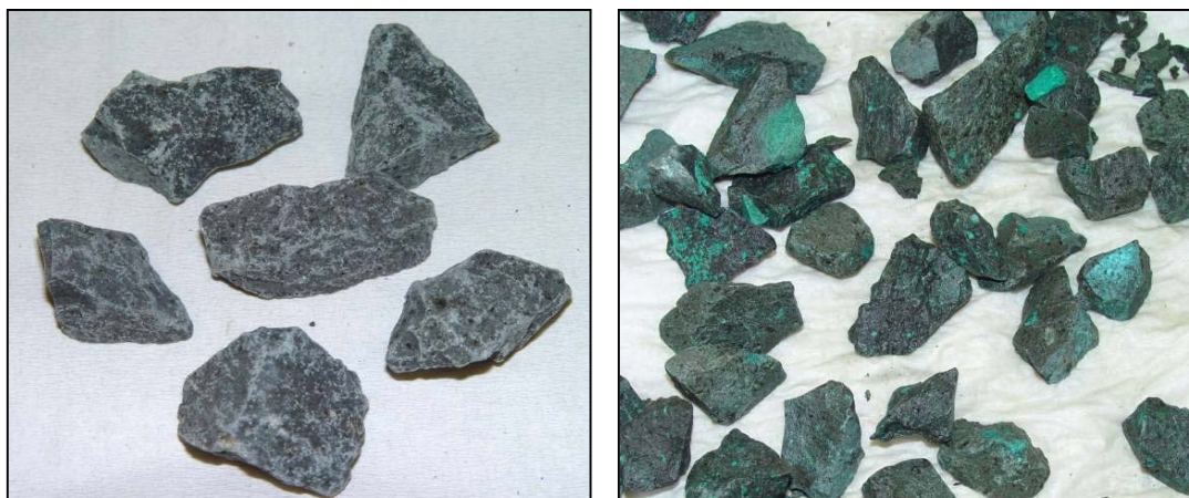
Figure 79. Venetia K2 West kimberlite unweathered (left) compared to the weathered product (right). Weathering was done in a 0.05 M cupric sulphate solution for 6 days.
