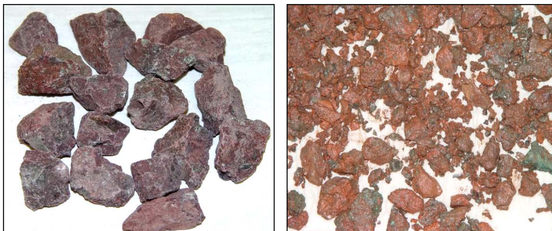
Figure 81. Venetia Red kimberlite unweathered (left) compared to the weathered product (right). Weathering was done in a 0.05 M cupric sulphate solution for 6 days.
