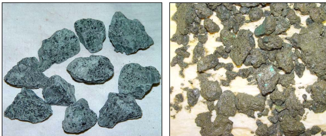
Figure 76. Venetia K1 TKB East kimberlite unweathered (left) compared to the weathered product (right). Weathering was done in a 0.05 M cupric sulphate solution for 6 days.
