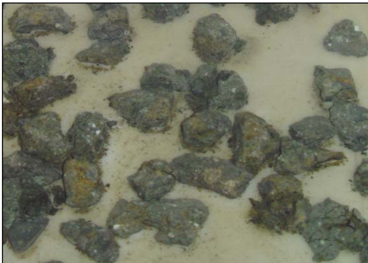
Figure 40. Visual appearance of Dutoitspan ore (initial size - 26.5 + 22.4 mm) weathered in lithium chloride solution (0.4 M) for 6 days.
