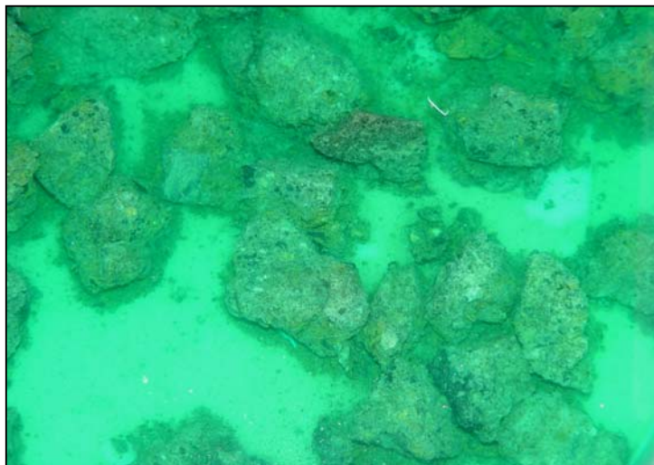
Figure 54. Visual appearance of Dutoitspan ore (initial size - 26.5 + 22.4 mm) weathered in cupric sulphate solution (0.2 M) for 12 hours.
