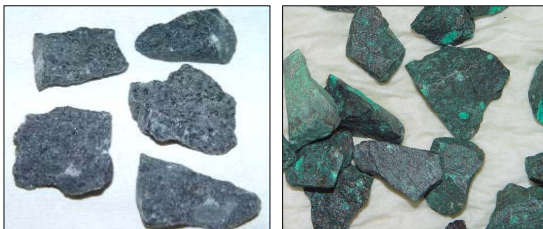
Figure 74. Venetia K1 Hypabyssal North East kimberlite unweathered (left) compared to the weathered product (right). Weathering was done in a 0.05 M cupric sulphate solution for 6 days.
