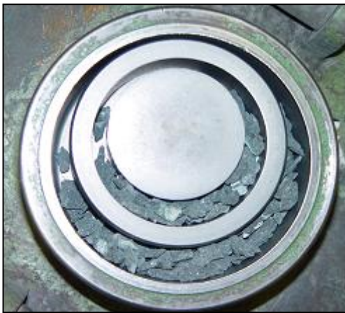
Figure 19. Ore added to the swing mill container for the agglomeration test showing the grinding metal pieces inside the container.
