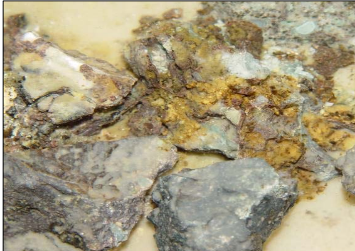
Figure 37. Visual appearance of Geluk Wes ore (initial size -22.4 + 19 mm) weathered in lithium chloride solution (0.2 M) for 6 days.
