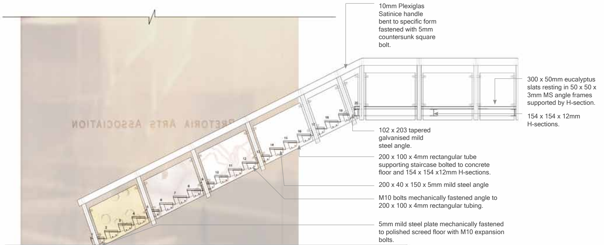
Fig. 5.4.14 NORTHERN ELEVATION_ STAIRCASE Scale 1 :50
