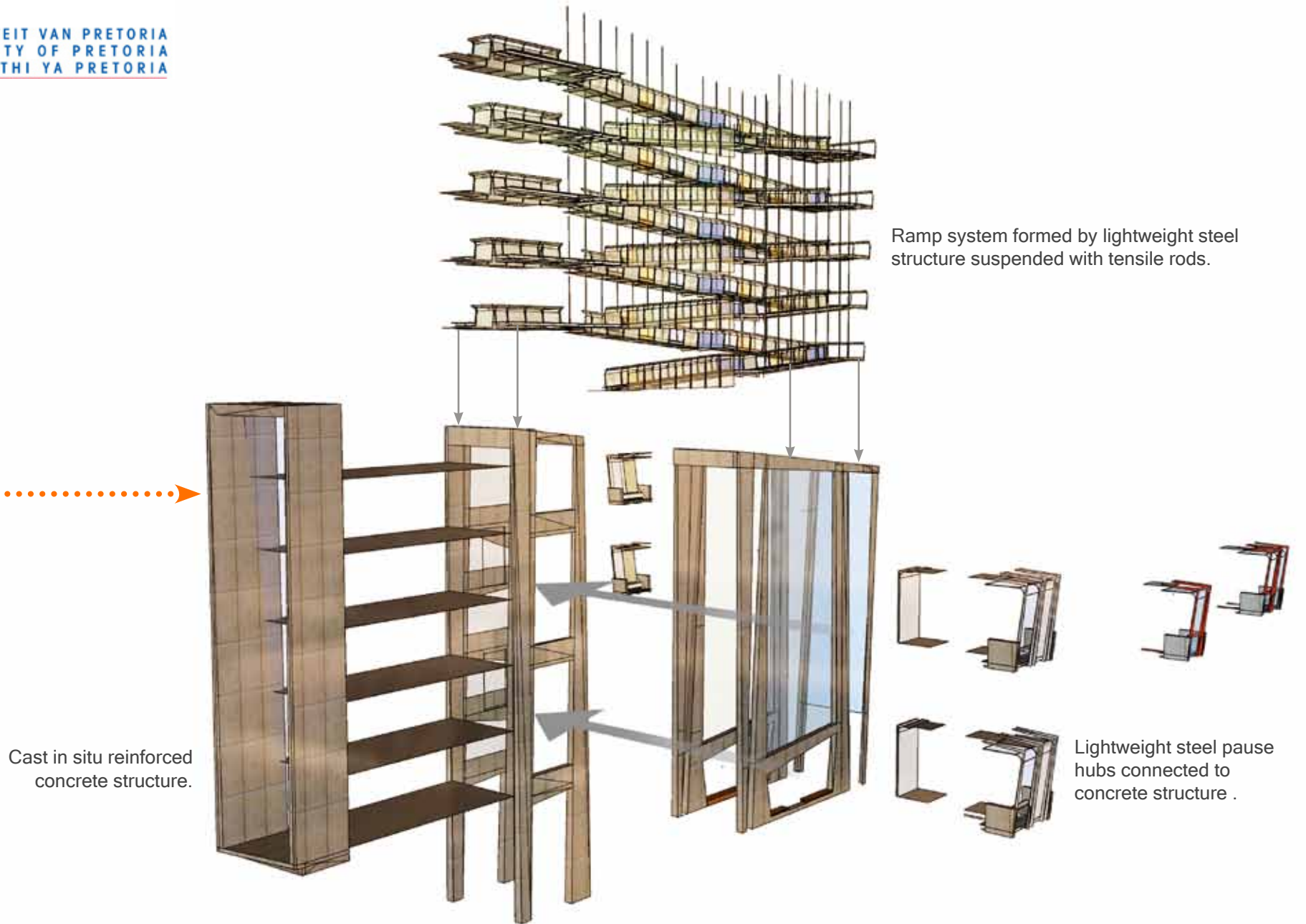
Fig. 5.4.3 Axonometric diagram of the additional vertical circulation core.
