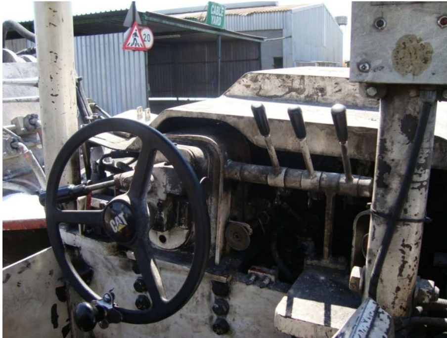
Figure 27. The driver's cabin, which is laid out perpendicular to the vehicle's heading.
