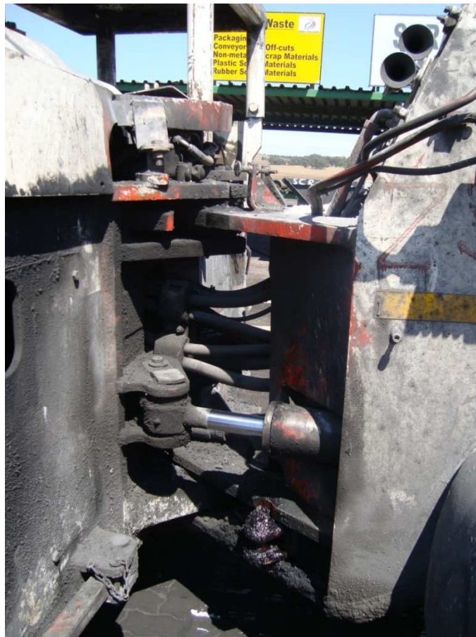
Figure 4. The articulation joint of a Wright 356B LHD.
