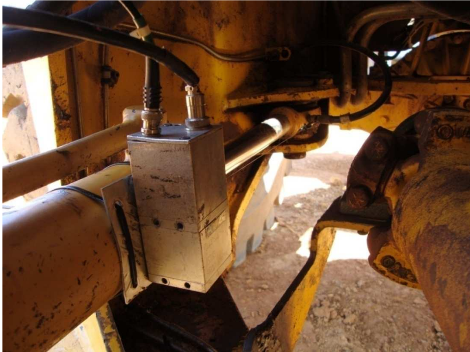
Figure 31. Placement of the rope displacement sensor.
