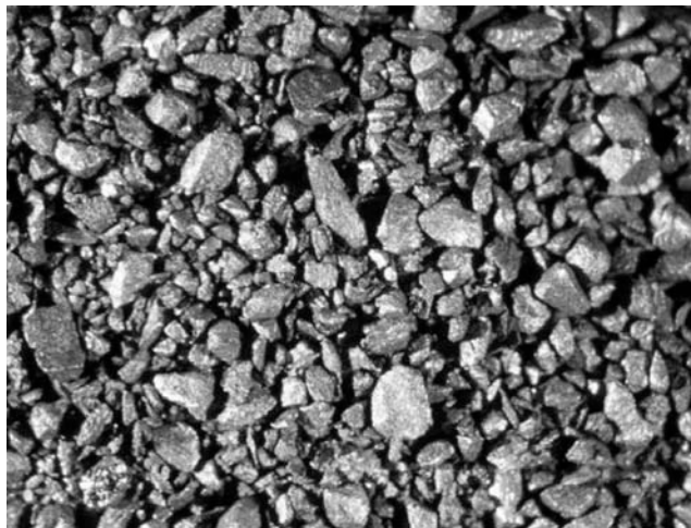
Figure A1.4: Residual char removed during magnetic separation (Approx. x10 magnification)
