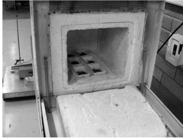
Figure 4.2: Sample containers arranged inside the furnace
