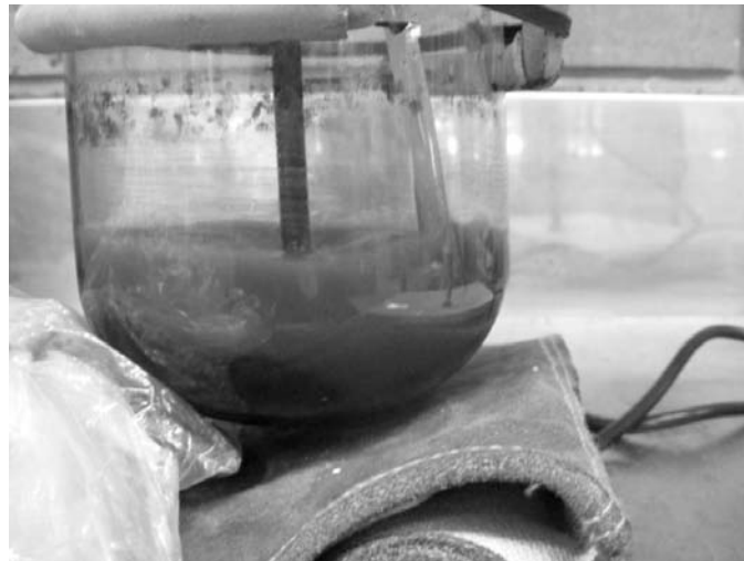
Figure A2.3: Mixing vessel to simulate “light” wet milling of nitrated ilmenite
