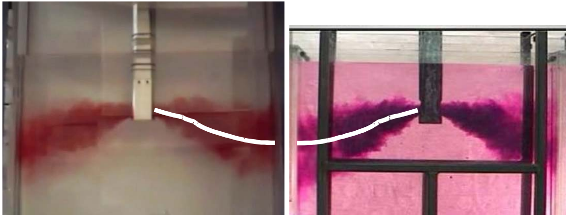
Figure 3.13: Comparison between full-scale ADVENT water model [32] and the 40%-scaled model, satisfying Fr-similarity in the latter case: 1060mm mould width
