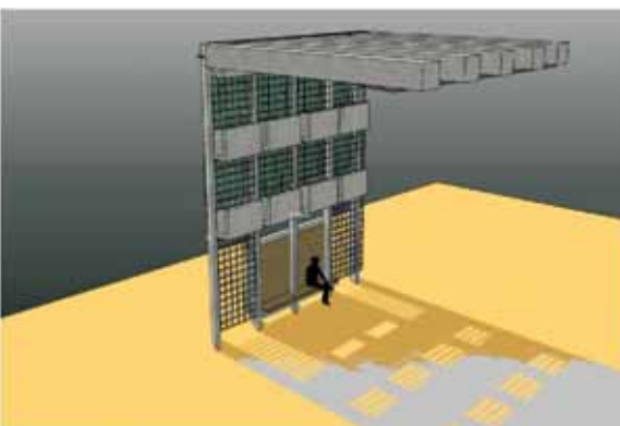
5_78 Concrete brise soleil , simulation of noon shadow projection, winter
