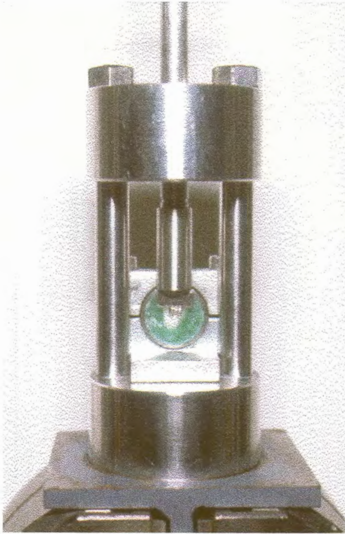
Figure 8: The SBS components of the Bencor Multi-T system contains a knife-edge guillotine for standardised positioning during force application on the bracket
