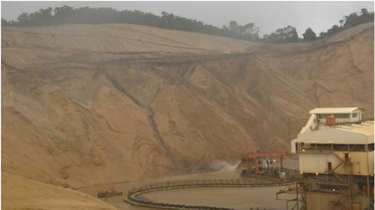
Plate 2. The mine works as an open-cast dredging system whereby dune sand is taken up by a bucket wheel and separated from the heavy minerals (~4% of the sand) by means of a cyclonic system on the mining plant. This heavy mineral concentrate is taken to the smelter site for further processing where the rutile, zircon and ilmenite are further separated and prepared.
