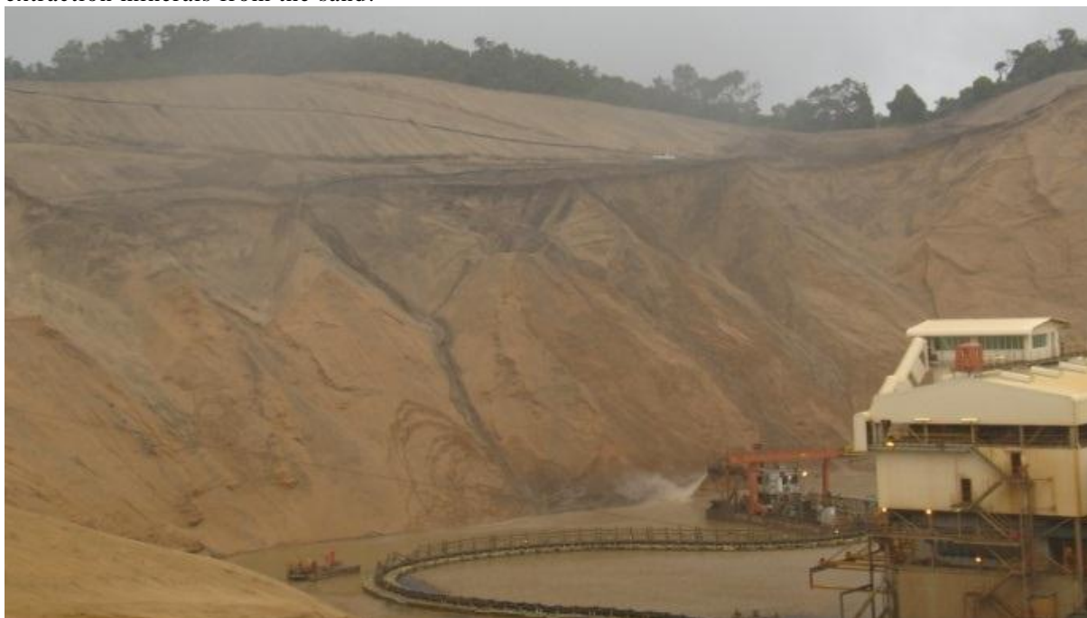
Plate 2. The mine works as an open-cast dredging system whereby dune sand is taken up by a bucket wheel and separated from the heavy minerals (~4% of the sand) by means of a cyclonic system on the mining plant. This heavy mineral concentrate is taken to the smelter site for further processing where the rutile, zircon and ilmenite are further separated and prepared.
