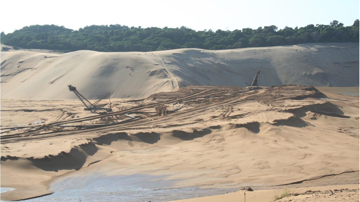
Plate 3. Once separated from the heavy minerals, the sand is stacked into shapes that mimic the pre-mining topographic profile.
