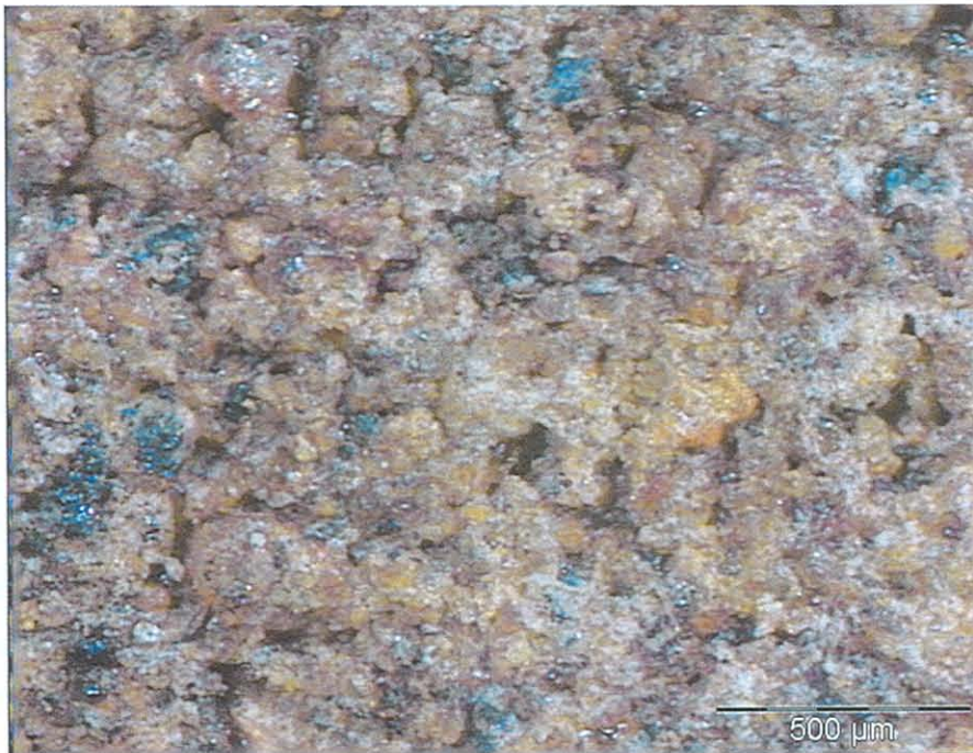
Figure 5.13 Sample from laboratory (2 % cement, 1.8 % net bitumen), 32x magnification
