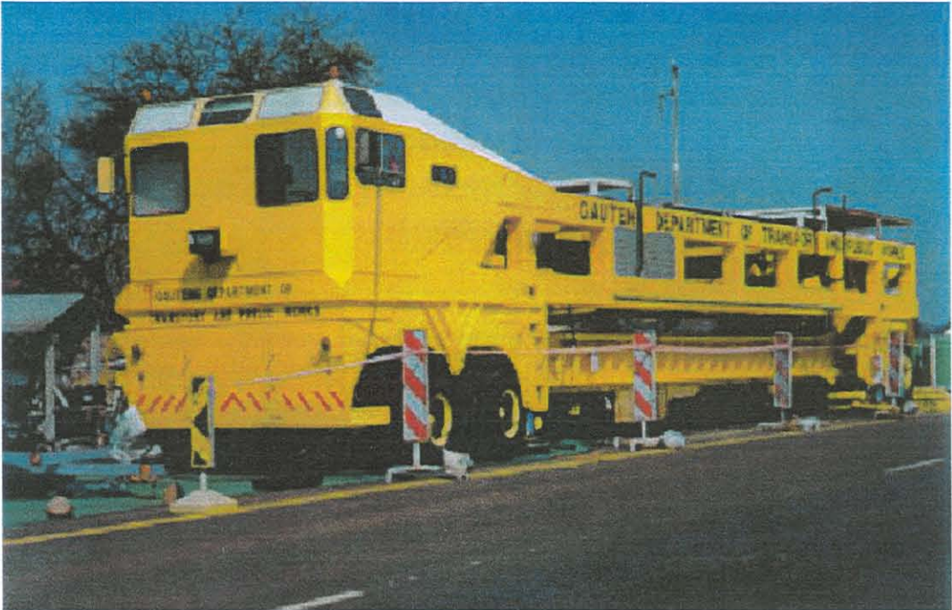
Figure 5.5 Overall view of the Heavy Vehicle Simulator
