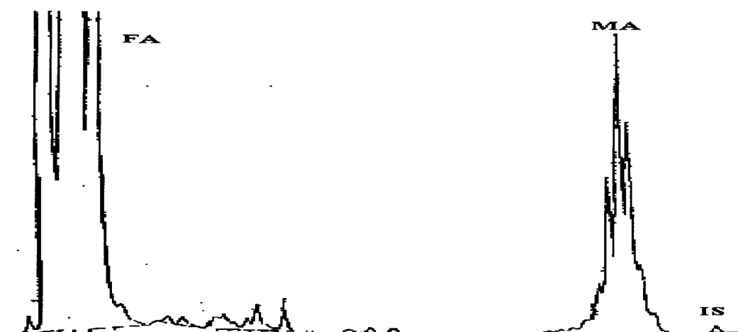
Fig.2.3: The HPLC profile of mycolic acids crude extract after funnel extraction. Crude extract was funnel-extracted twice with equal volumes of lower phase and the upper phase. FA represents the derivatised fatty acids peak, MA represents mycolic acids peak and IS represents the internal standard peak.
