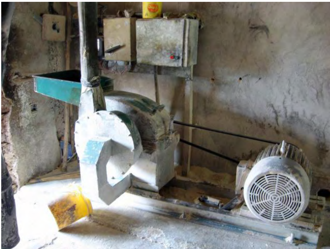
Figure 3.11: The electrical hammer mill popularly known as the “Posho mill” which is used for milling sorghum grain into flour (Picture courtesy of Prof. J.R.N. Taylor)
