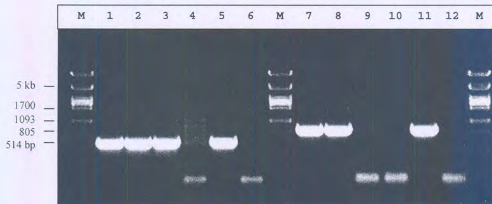
Figure 4.2 Colony PCR of A. tumefaciens GV3101 using AP-PGIP and NPTII primers. M: λDNA/ PstI marker; lanes 1 to 3: NPTII PCR of colonies transformed with GSTI prom- apgip1 -pCAMBIA#30, pCAM2300- apgip1B and pCAMBIA2300, respectively; lanes 4 to 6: NPTII PCR of untransformed A. tumefaciens GV3101, positive control and negative water control, respectively; lanes 7 to 12: AP-PGIP PCR with the same templates as the NPTII PCR.
