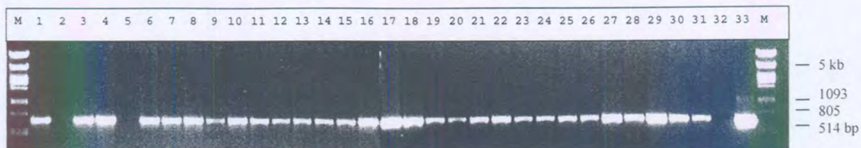
Figure 5.2 nptII PCR with gDNA from in vitro transgenic potato leaf material. M: \lambda DNA/ Pst I marker; lane 1: LA Burley: pgip1 #8 positive control; lane 2: untransformed LA Burley negative control; lanes 3 to 31: putative transgenic potato lines A2, A3, A4, A5, A6, A7, A8, A9, A10, A11, A12, A13, A14, 7A, B1, B2, B3, B4, B5, B6, B7, B9, B10, B11, B12, B13, B16, B17 and B18, respectively; lane 32: negative water control; lane 33: positive control with plasmid as template.
