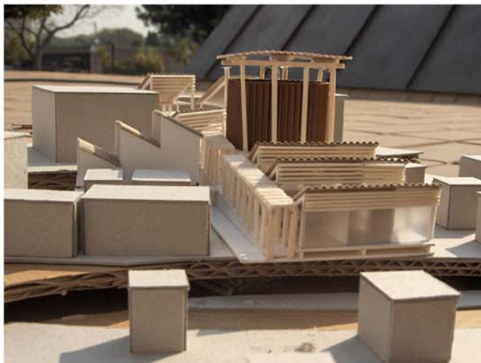
FIG. 220: 1:200 WORKING MODEL SHOWING THE PRELIMINARY CONCEPT FOR THE EMPOWERMENT CENTRE WITH EAST-FACING SAWTOOTH ROOFS - EAST CORNER (AUTHOR, 2006).
